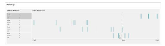
The shaded bars show the workload scores for individual virtual machines in each round. A light, dotted line shows the average score for all active clients in the round.
